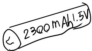
$$\begin{aligned}Q_{\max} &= 2300 \text{ mA} \cdot \text{h} \\ &= 2300 \text{ mA} \cdot (3600 \text{ s}) \\ &= 2300 \times 10^{-3} \times 3600 \text{ C}\end{aligned}$$
