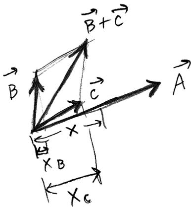
$$\begin{aligned} \vec{A} \cdot (\vec{B} + \vec{C}) &= xA = (x_B + x_C)A \\ &= x_B A + x_C A = \vec{A} \cdot \vec{B} + \vec{A} \cdot \vec{C} \end{aligned}$$
