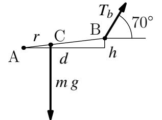
$$\begin{vmatrix} r \cos \theta & r \sin \theta \\ 0 & -mg \end{vmatrix} + \begin{vmatrix} d & h \\ T_b \cos(70^\circ) & T_b \sin(70^\circ) \end{vmatrix} = -mg r \cos \theta + T_b (d \sin(70^\circ)) - h \cos(70^\circ) = 0$$
