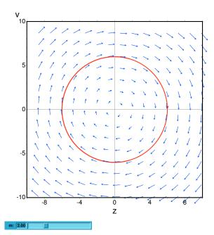
• To plot the direction field of the Duffing equation,  $m*x''+c*x'+k*x+b*x^3=0$ , we introduce the variable y=x' and use:
