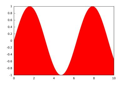
Region bounded by an explicit object and the function defined by option filled\_func. Note that the variable in filled\_func must be the same as that used in explicit.
