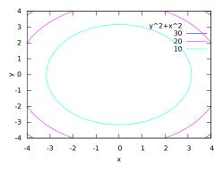
You can add any options accepted by plot3d; for instance, the option legend with a value of false, to remove the legend. By default, Gnuplot chooses and displays 3 contours. To increase the number of contours, it is necessary to use a custom gnuplot\_preamble, as in the next example:
