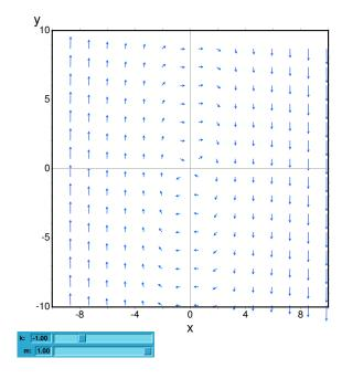
• The direction field for a damped pendulum, including the solution for the given initial conditions, with a slider that can be used to change the value of the mass m, and with a plot of the two state variables as a function of time:
