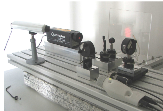
Figure 2. Michelson Interferometer – current stage
